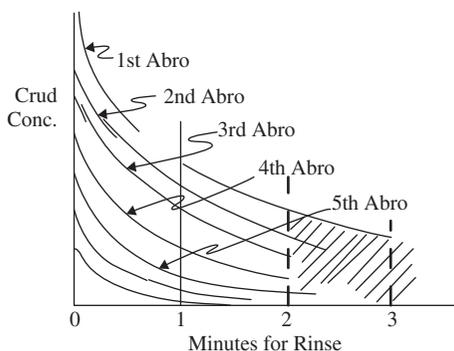
Abro in the external regeneration tank (Air Bump Rinse Operation).
