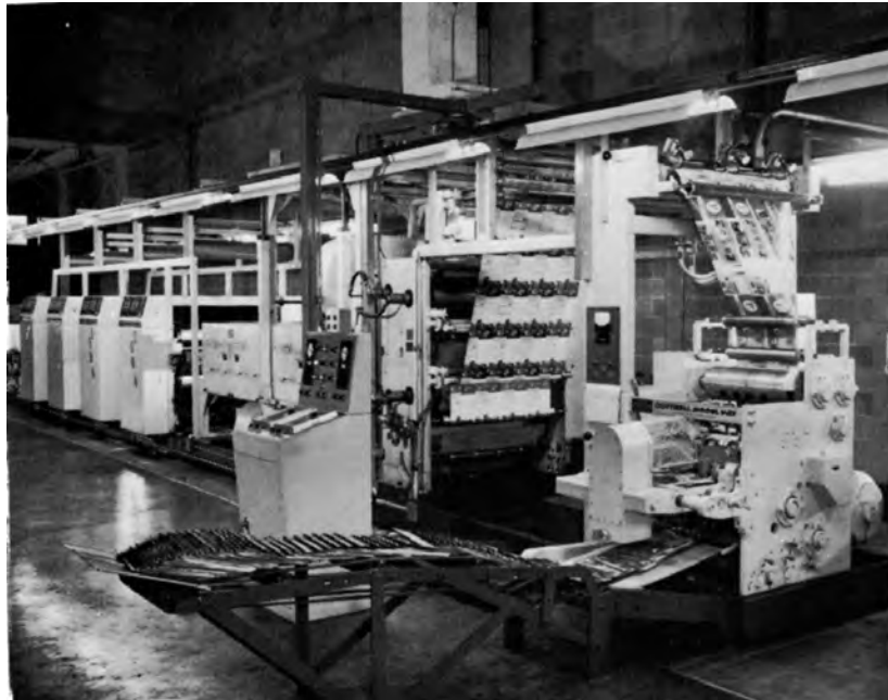
Fig. 1-6. Cottrell Model V-22 newspaper press ( Courtesy of The Cottrell Co., Division of Harris-Intertype Corp. ).
